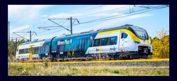
With Mireo Plus H, Siemens Mobility is continuing the Mireo success story. This hydrogen train is the smart alternative to diesel multiple units and a trailblazer for emission-free operation on long-distance routes without an overhead contact line. At the same time, it features all the qualities of Mireo, including energy efficiency, a flexibly adaptable interior design, and low maintenance and lifecycle costs.
