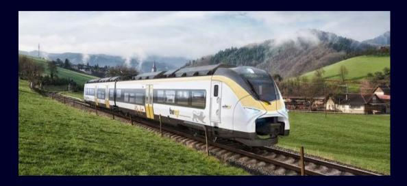
The Mireo Plus B battery hybrid train features operation that is extremely cost- and energy-efficient as well as locally emission-free. This makes it ideal for modern, European regional transport as a smart alternative to conventional diesel multiple units, especially on non-electrified or only partially electrified lines.
